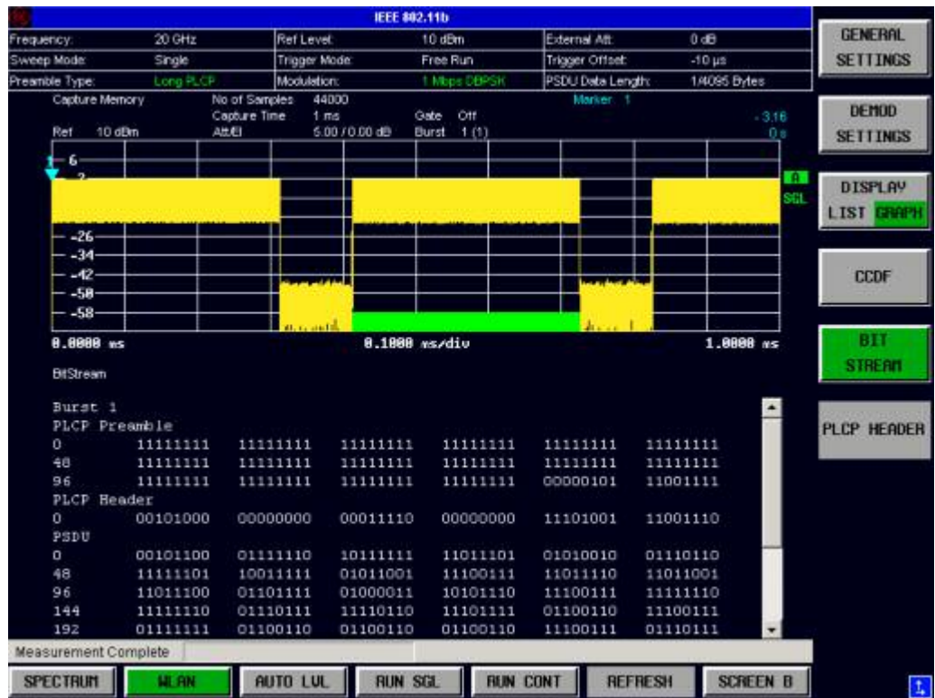
Fig. 2-18 IEEE 802.11b & g (Single Carrier) Bit-Stream Results
